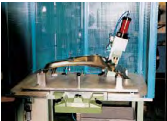
Device for holes Ø 8 in sheet metal
