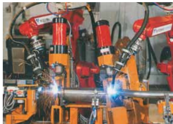
Welding fixture for exhaust components
